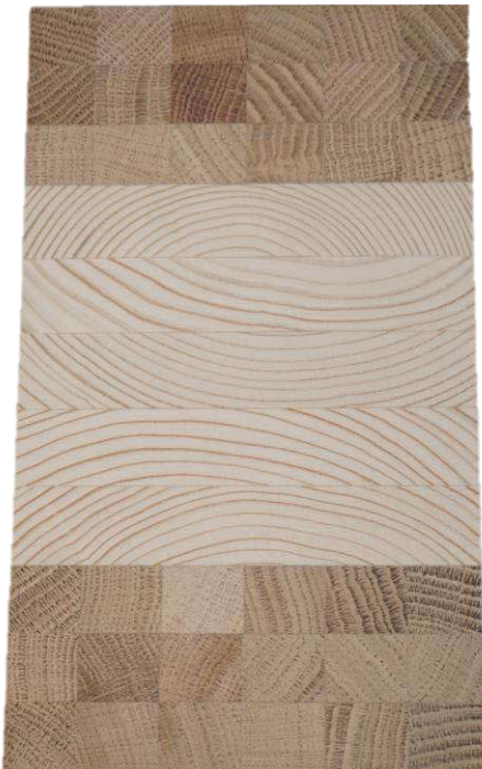
Production of hybrid GLT layups with oak/ beech Strip-like laminations
